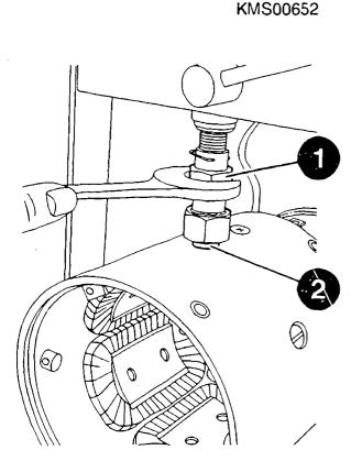
REPLACING EXCITATION WINDING
